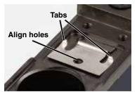
Place the spring detent clip on the housing with the tabs facing upward and the screw hole aligned with the one in the housing.
